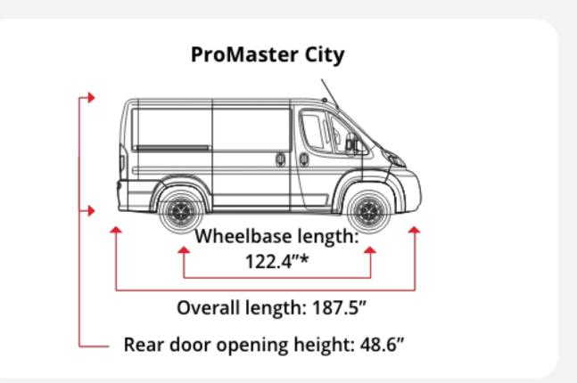
\*Wheelbase is measured from the center of the front wheels to the center of the back wheels.
